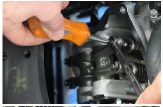
Check the correct sliding and the presence of axial play of the decompression mass during the entire excursion with the engine at the TDC (absence of jamming).
