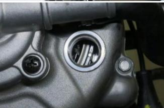
Check the correct valve clearance (Intake
