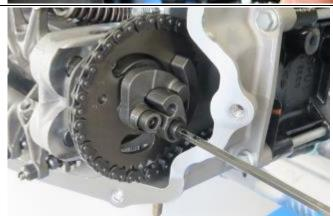
4. Check the correct combination of the camshaft and the decompressor classes (A-A, B-B, C-C).
